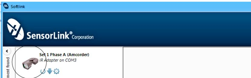
The description and photo displayed will change from the communication device to the unit when the Recorder has been discovered.
