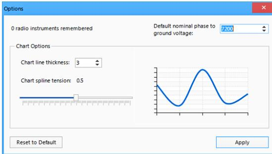
**Chart line thickness:** The thickness of the graph lines can be changed by the user. Thickness is numbered 1 - 10, and defaults at three. The software will show a preview to the user as the value is changed.
