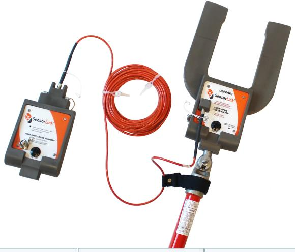
The Amp Litewire is a True RMS high voltage rated ammeter designed to measure True RMS curent on the primary side of a distribution network. The sensor probe is attached to an insulated hot stick and positioned onto the medium or high voltage line. A fiber optic cable connects the sensor probe to a receiver unit at ground potential, which delivers the current waveform measurement as an analog output to a meter analyzer.
