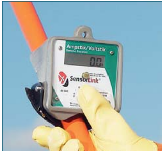
Receiver Display on Hotstick
