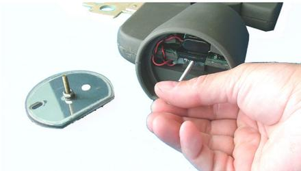
3. Adjust the hexnut, located on the bottom of the standoff assembly shaft, as needed, to set the overall height of the standoff to approximately 1-1/2".
