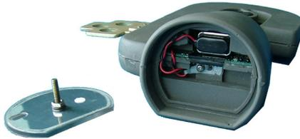
2. Screw the male end of the standoff assembly into the threaded hole.
