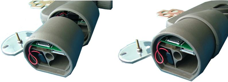
7. Place the front panel assembly onto the the Radio Transcorder and turn the thumb screw to tighten. Do not over tighten.
