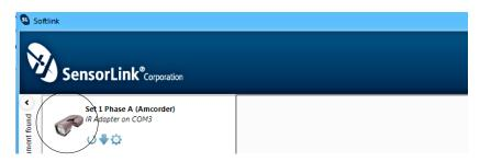
The description and photo displayed will change from the communication device to the unit when the Recorder has been discovered.
