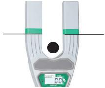
**Step 5:** Hold the unit on the conductor for 2-4 seconds and then remove from the line. The measurement has been taken and the unit is ready to take the next reading. Each reading is numbered and displayed on the top left of the display.
