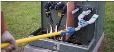
Overhead current measurement Ampstik®+, Model 8-020-XT PLUS, Standard Sensor Opening
